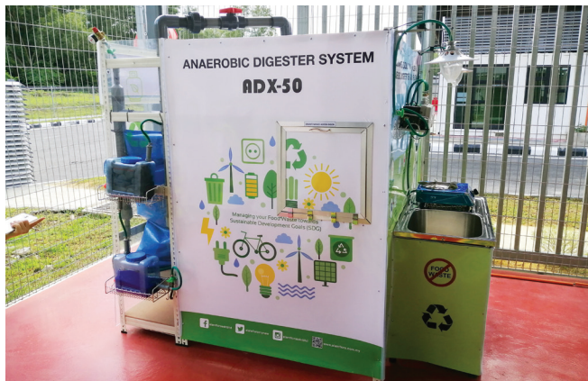
The smaller 50kg AD machine is also available for use at individual premises.
