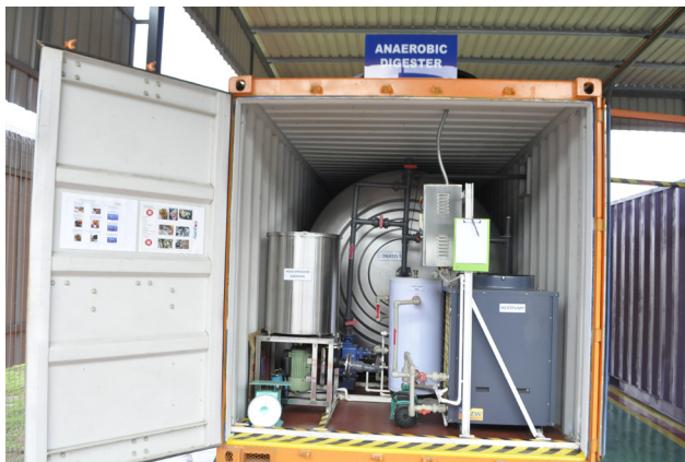
This AD machine with 500kg capacity can produce biogas and biofertilizers as a result of the food waste decompose process.
