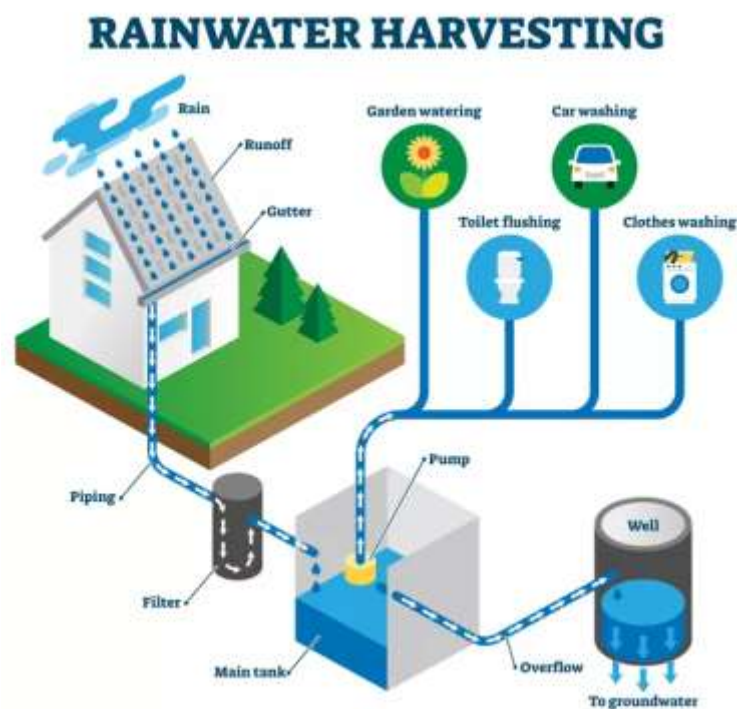
Figure 29: Rainwater harvesting system with hose roof water runoff, underground piping, filtering, collecting in tank for domestic use.
